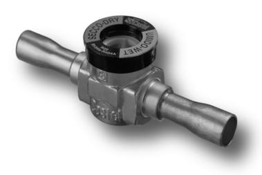
element from green fade to yellow, "green Chartreuse", working conditions of the system could become difficult. When the sensitive element becomes "yellow", it's time to substitute the dehydrator filter. If the charge and working condition are normal, the refrigerant fluid appears perfectly liquid underneath the "lens" of the indicator. The presence of bubbles indicates that the refrigerant fluid is partial evaporating along the liquid line.
